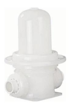
Micropore PP Filter Housing 226 type is made of PP, PVC materials which have good chemical compatibility. Simple configuration design makes the installation and operation easier. The housing is designed to fit 10'' 334 single open end cartridge. The material used is safe and low precipitation. It can be used in the filtration of water and general chemicals in kinds of industry.
